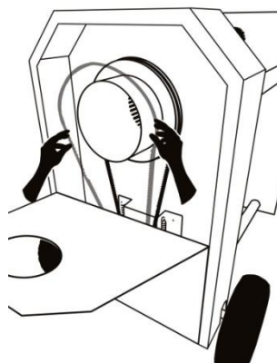
2.Remove the drive belt by pulling it up
