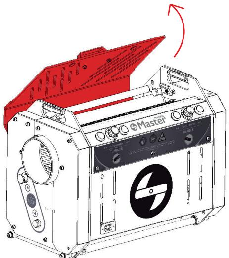
**8** Pull the 2 positioners towards the inside and rotate them 90° to separate the two parts of the trimmer (A) and remove the front part (electrical module) with the handles.
