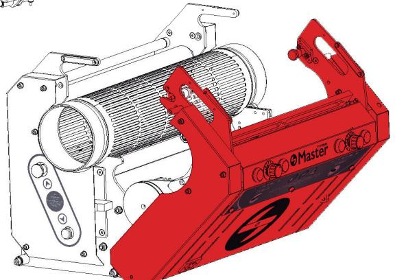
**10** Remove the blade. Pull the two positioners out and turn them 90°. Hold the blade carefully and remove it from the machine. (Make sure that the blade is in a good condition. If it is bent, twisted or if it has some scratches you should change the blade. Otherwise it could damage the machine).
