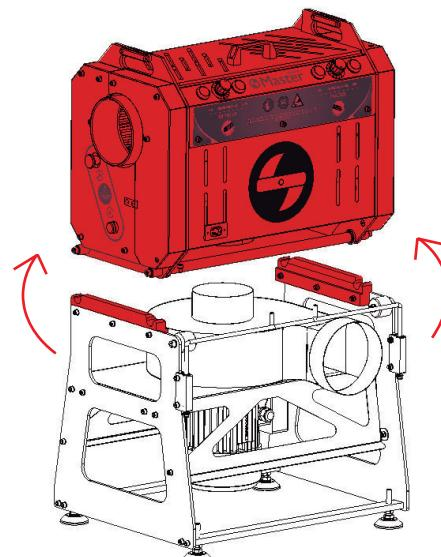
**7** Remove the top cover with the help of the handle.
