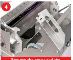
Remove the cover and the electrical assembly.
