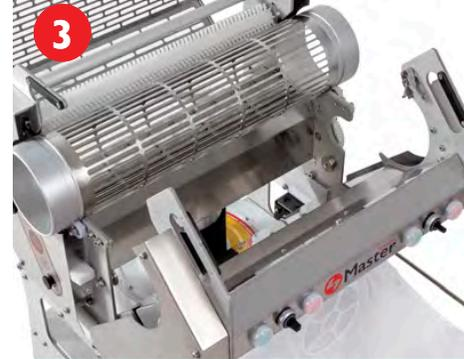
Open the trimmer and remove the barrel.
